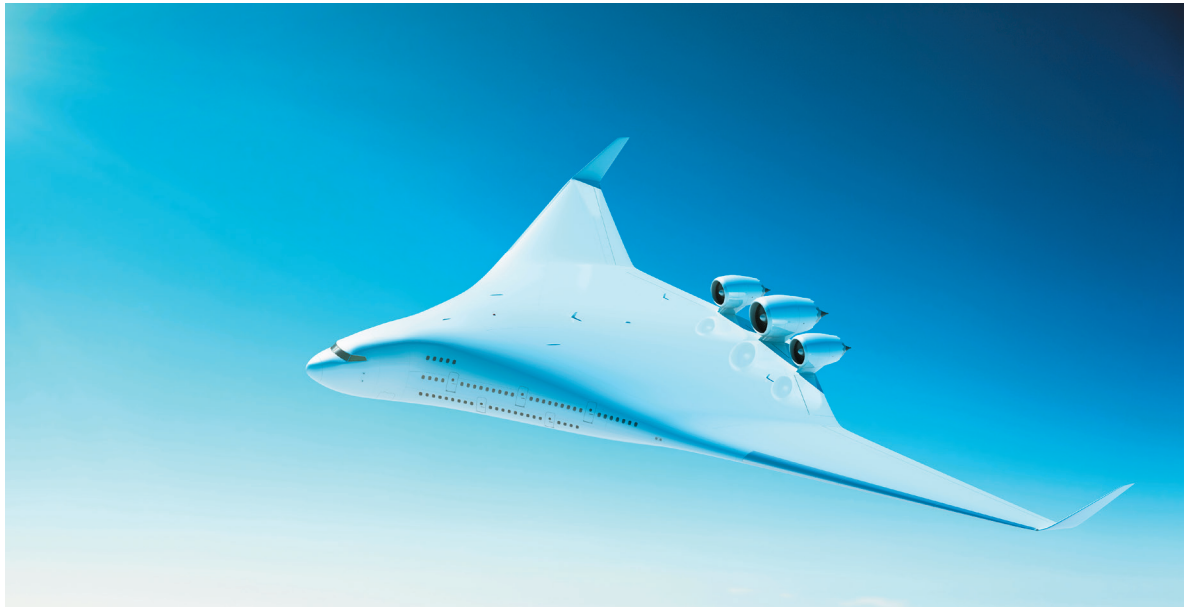
Figure 2. The increased fuselage space of blended wing body aircraft can be used to store batteries, hydrogen or hydrogen and fuel cells without sacrificing passenger or cargo capacity.
