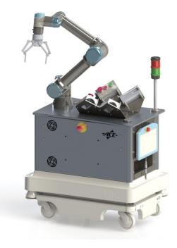
and wheel-based load carriers that travel along the floor of a facility without an onboard operator or driver, guided by a combination of software and sensor-based guidance systems. AGVs provide the safe movement of cargo by following a predictable course. Both can encounter an unexpected obstacle while navigating their environments, such as a fallen box or a crowd of people.
