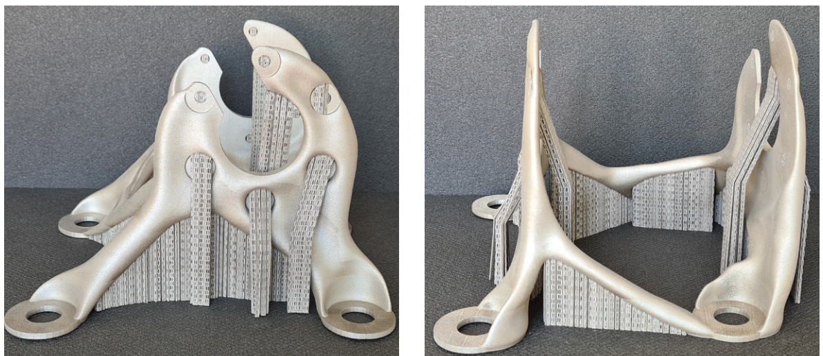
Figure 9. Bracket printed with nominal print strategy and supports (as reference).
