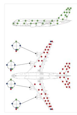
The Airbus Flutter team in Toulouse performed a variety of excitations, including control surfaces sine sweeps and pulses. Pulses are currently used to assure crew and aircraft safety, whereas sweeps are used to work out more accurate results, enabling the update of theoretical finite element (FE) models. Thanks to integrating pulses into the process, the duration of flutter flights has been considerably reduced.
