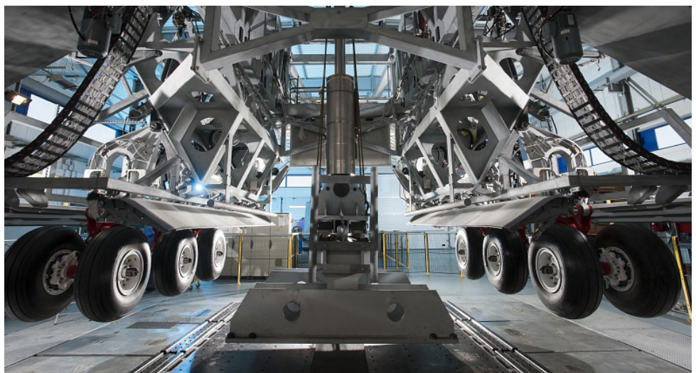
A400M landing gear systems test rig
