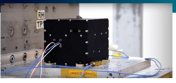
In the test phase, the bulletshot by the air gun excites the ringing plate, and a special pyroshock accelerometer transmits the response signals to the Siemens Simcenter SCADAS mobile data acquisition hardware. The obtained response signals are then analyzed using Siemens' Simcenter Testlab software.
