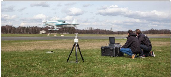
Impact of electric propulsion estimated with a flyover noise measurement setup.
