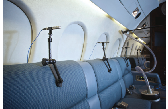
The transfer path analysis technique helps find the root cause of noise and vibration issues (image courtesy of Belgian Defense Forces).
