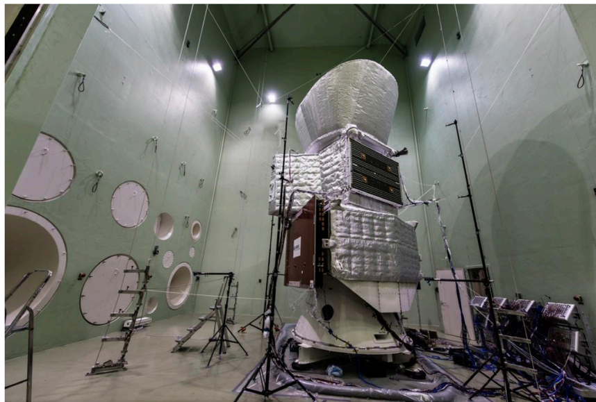
Figure 9. Reverberant field acoustic excitation test at the European Space Agency (ESA).
